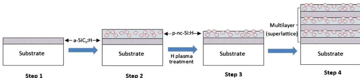
**Fig. 1.** The detailed deposition process of p-nc-Si:H/a-SiC<sub>x</sub>:H QDSL samples (1) a single a-SiC<sub>x</sub>:H layer and (2) p-nc-Si:H layer, (3) H plasma treatments, and (4) a multilayer structure.
