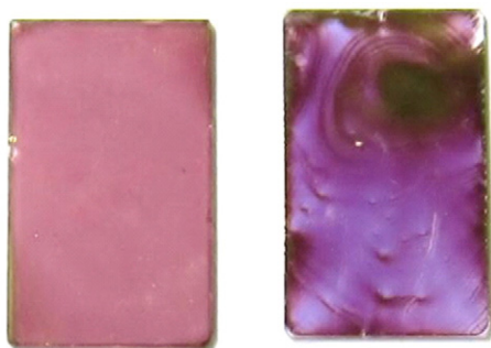
Fig. 1. (Color online) Photographs of P3HT (left) spin-coated and (right) drop-cast thin films fabricated in a dry N_2 atmosphere onto quartz substrates that were preliminarily baked to remove adsorbed water.
