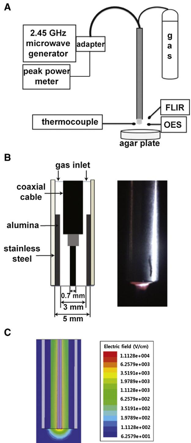
Fig. 1. Overview of microwave plasma jet device. A. Schematic view of a microwave generation system. B. Schematic view (left panel) and picture (right panel) of microwave plasma jet device. C. Electrical field generated in the vicinity of plasma source.
