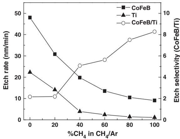
**Fig. 1.** Etch rate of CoFeB films and Ti hard mask, and etch selectivity of CoFeB to Ti films at different CH<sub>4</sub> concentrations in the CH<sub>4</sub>/Ar gas; etch condition: ICP rf power of 800 W, dc-bias voltage of 300 V, and gas pressure of 0.67 Pa.
