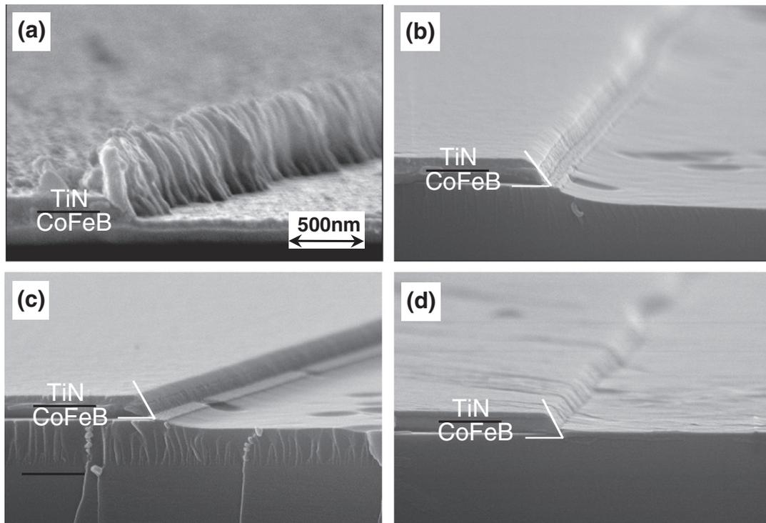
**Fig. 2.** FESEM micrographs of CoFeB films etched using (a) pure Ar, (b) 40% CH<sub>4</sub>/Ar, (c) 60% CH<sub>4</sub>/Ar, and (d) 80% CH<sub>4</sub>/Ar; etch condition: ICP rf power of 800 W, dc-bias voltage of 300 V, and gas pressure of 0.67 Pa.
