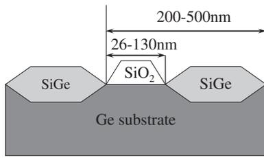
Fig. 1. A schematic cross-sectional view of the fabricated strained Ge structure with embedded SiGe stressors.
