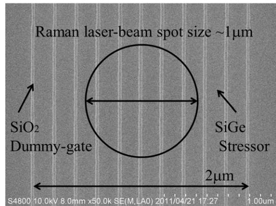
Fig. 4. A plan-view SEM image of SiO<sub>2</sub> dummy-gated strained Ge structures (*L/S* = 30/170 nm) with SiGe stressors with *x* of 0.7. Around 5 strained Ge channels are included in a Raman beam spot.
