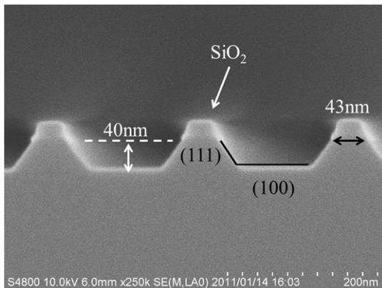
Fig. 2. A cross-sectional SEM image of Ge substrate recessed with HPM anisotropic etching.
