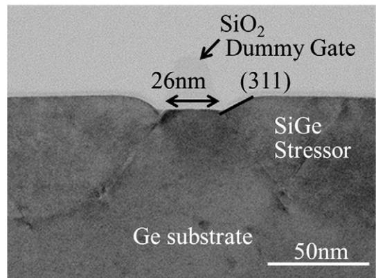
Fig. 3. A cross-sectional TEM image of 26 nm SiO<sub>2</sub> dummy-gated strained Ge structures with SiGe stressors with *x* of 0.7.
