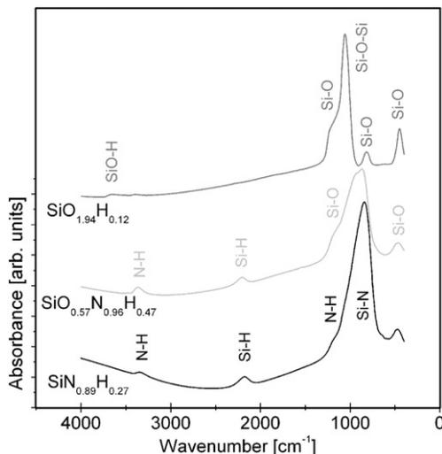
Fig. 1. FTIR absorption spectra of silicon oxide, oxynitride and nitride. The assigned bonds are provided in the figure.
