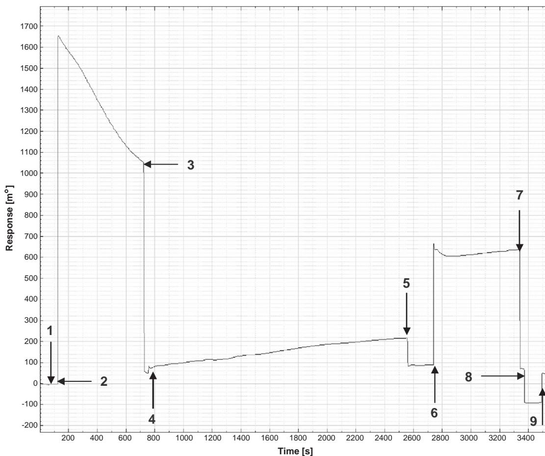
**Fig. 1.** Sensorgram showing different steps [(1) Baseline, (2) EDC-NHS activation, (3) Washing, (4) Antibody coupling, (5) Washing, (6) Deactivation, (7) Washing, (8) Regeneration and (9) Back to baseline] involved in the immobilization of SEB antibody (1 ng/ml) on the carboxymethyl dextran modified gold chip.
