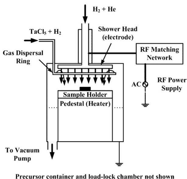
Fig. 1. Schematic diagram of PACVD reactor.
