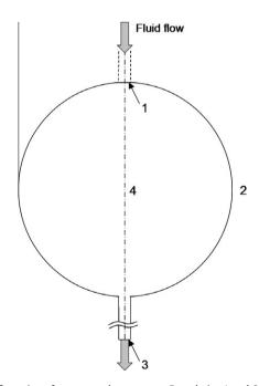
**Fig. 1.** Configuration of an open-sphere system. Boundaries 1 and 3 indicate the inlet and outlet, respectively. Boundary 2 is the vessel wall, and boundary 4 is the axis of symmetry.
