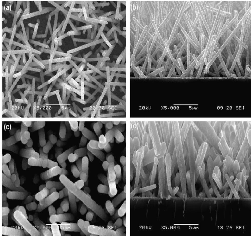
Fig. 2. SEM images of the Co<sub>3</sub>O<sub>4</sub> nanorods: (a) top view and (b) cross-section view; SEM images of the Al/Co<sub>3</sub>O<sub>4</sub> nEMs: (c) top view and (d) cross-section view.
