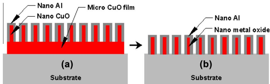
Fig. 1. Sketch of nEMs composed of: (a) nanofuel and nano/microscale oxidizer, and (b) nanofuel and nanooxidizer (no microscale oxidizer).
