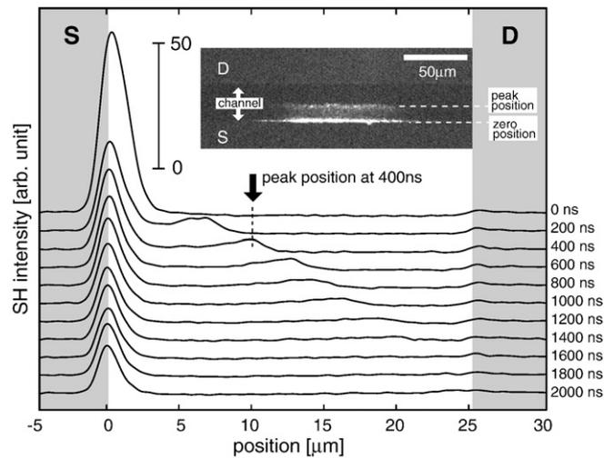
**Fig. 2.** Change in the SHG intensity distribution under a positive pulse application to the Ag source electrode. The inset is an actual SHG image from the OFET channel. For the SHG intensity distribution, the origin of the x-axis is set to the edge of source electrode ( $x = 0$ ). Peak position of the SHG distribution at 400 ns is also indicated by black arrow as an example.
