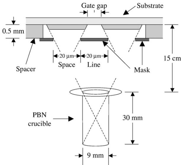
Fig. 2. Evaporation process.
