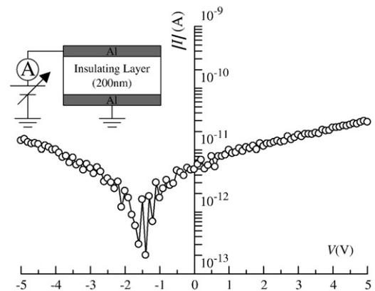
Fig. 4.  $I$ – $V$  characteristics of insulating layer.
