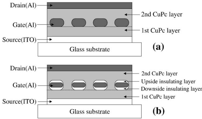
Fig. 1. OSIT structure (a) without insulating layer (b) with both sides insulating layers.
