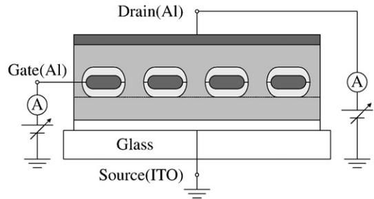
Fig. 3. Measurement system for static characteristics.
