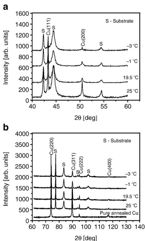
**Fig. 1.** XRD patterns of copper films prepared by sonication at different temperature at low and high  $2\theta$  values.
