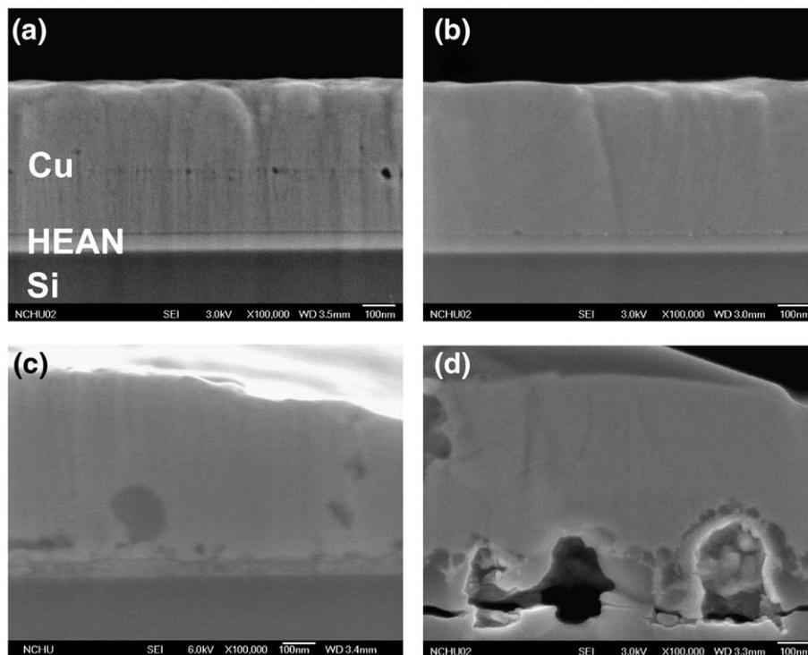
Fig. 1. SEM cross-sectional microstructures of Si/AlCrTaTiZr HEAN/Cu film stacks, (a) as-deposited, and after thermal annealing at (b) 700 °C, (c) 800 °C, and (d) 900 °C for 30 min.
