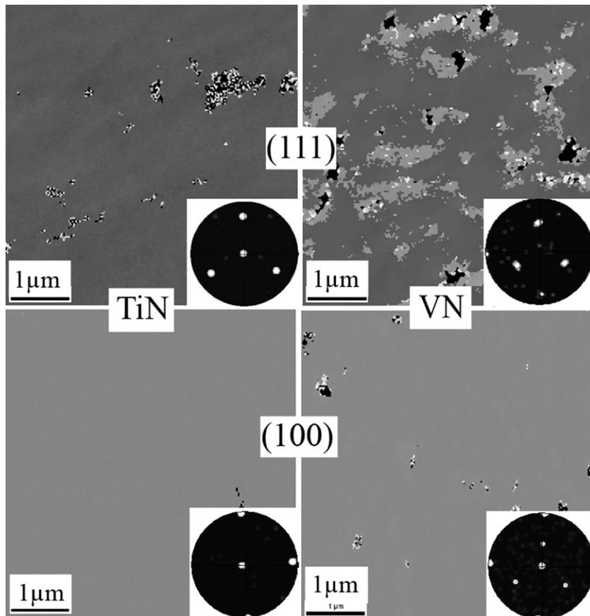
Fig. 2. EBSD analyses (scanned area of  $5 \times 5 \mu\text{m}^2$ ) and (001) pole figures (large area scan of  $850 \mu\text{m}^2$ ) of TiN and VN films grown on MgO (100) and (111) substrates.
