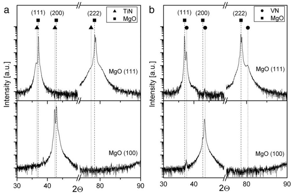
Fig. 1. XRD patterns of (a) TiN and (b) VN films grown on MgO (100) and (111) substrates.
