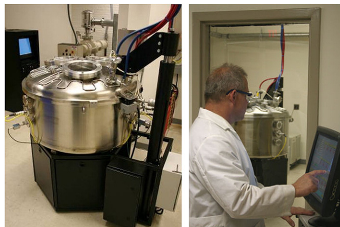
Fig. 2. GVD's 40 in. x 20 in. commercial iCVD coating tool. This system is currently used to deposit PTFE coatings, but can be adapted for deposition of many other iCVD polymer coatings, as needed.
