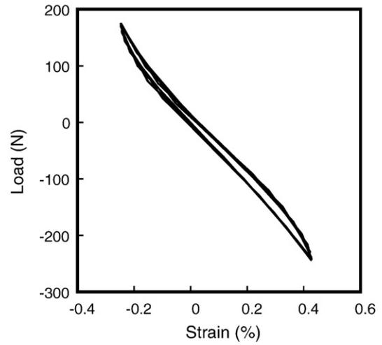
Fig. 1. Load versus strain for five cycles of a fatigue test of an Au/PC specimen.
