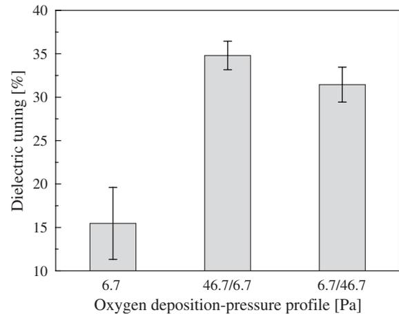
Fig. 2. Average percent dielectric tuning at 2 GHz for  $\text{Ba}_{0.6}\text{Sr}_{0.4}\text{TiO}_3$  1 mol% W-doped films deposited in different oxygen-pressure profiles.
