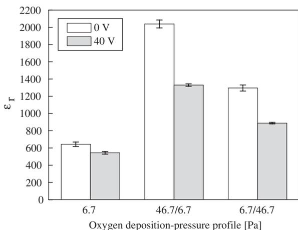
Fig. 1. Average dielectric constant at 2 GHz for  $\text{Ba}_{0.6}\text{Sr}_{0.4}\text{TiO}_3$  1 mol% W-doped films deposited in different oxygen-pressure profiles.
