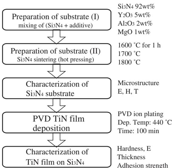
Fig. 1. The flow chart of synthesis of Si<sub>3</sub>N<sub>4</sub> substrates and deposition of the PVD TiN film on Si<sub>3</sub>N<sub>4</sub>.
