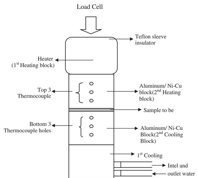
Fig. 1. Schematic diagram of experimental setup for both thermal and electrical resistance measurements.
