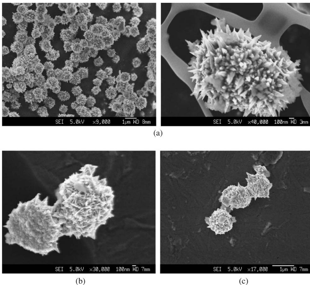
Fig. 2. FESEM micrograph of Ni particles prepared from Ni salt with different concentrations: (a) 0.05, (b) 0.025, and (c) 0.01 M.
