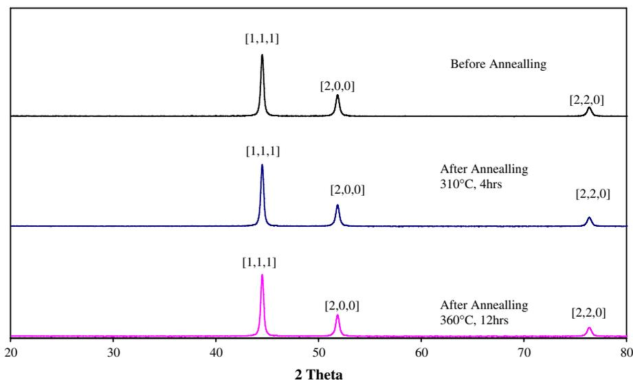
Fig. 3. XRD patterns of the Ni particles before and after annealing.
