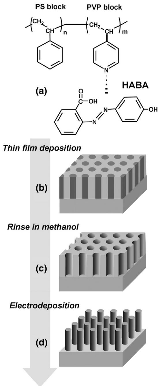
Fig. 1. The SMA based approach for metal nanorod array fabrication: chemical composition (a), microphase separation in thin films of SMA (b), nanotemplate (c), array of nanochannels/nanorods (d).
