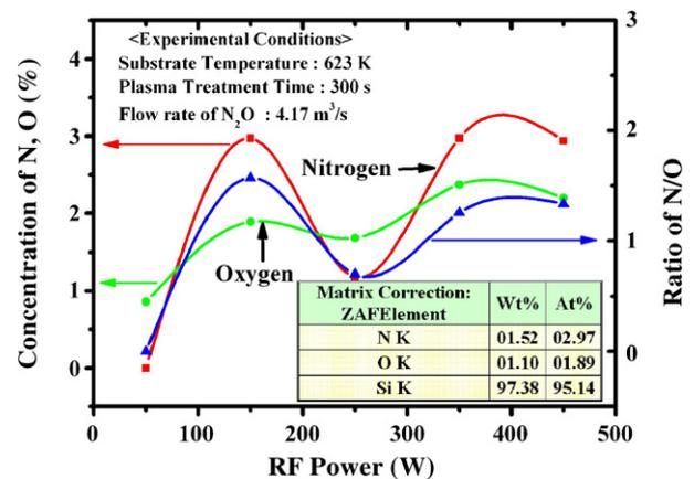
Fig. 3. Composition and EDS analysis of every ultra-thin SiO<sub>x</sub>N<sub>y</sub> films grown by varying RF power. The inset shows weight percentage and atomic percentage of the original spectrum obtained by EDS about the ultra-thin SiO<sub>x</sub>N<sub>y</sub> film fabricated by using RF power, flow rate of N<sub>2</sub>O, substrate temperature, and plasma treatment time of 150 W, 4.17 m<sup>3</sup>/s, 623 K, and 300 s.
