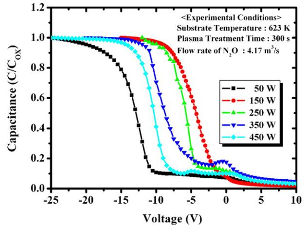
Fig. 2. The capacitance–voltage (C–V) characteristics of MOS structures using ultra-thin SiO<sub>x</sub>N<sub>y</sub> films grown by varying RF power as gate insulator. The electrical C–V measurements are performed by voltage sweep from inversion (+V) to accumulation (–V).
