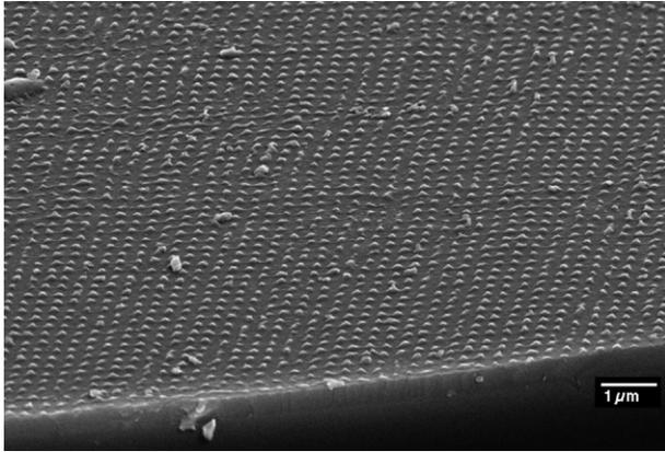
Fig. 1. SEM micrograph of the poly-Si surface crystallized by using ELA.
