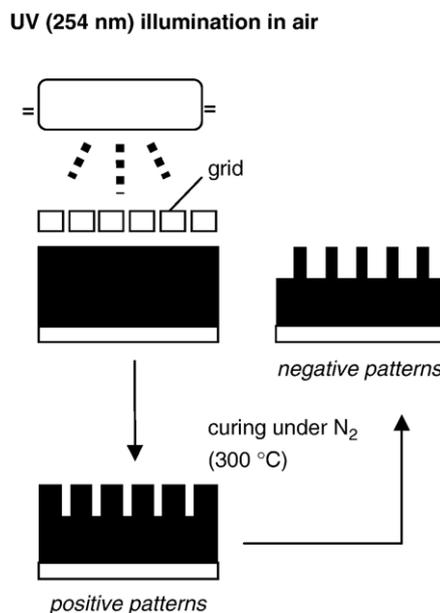
Fig. 1. Schematic procedure to prepare the PMSSQ films with positive and negative patterns.
