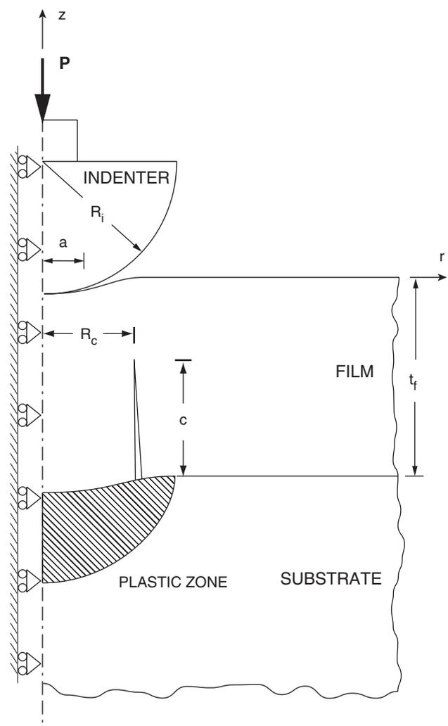
Fig. 1. Schematic of the model used in the fracture analysis. The illustration shows an axisymmetric section of a flexure induced transverse crack of length  $c$  emanating upwards from the interface at a radial location  $R_c$ .
