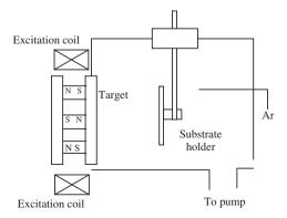
Fig. 1. Schematic diagram of the unbalanced magnetron sputtering system.
