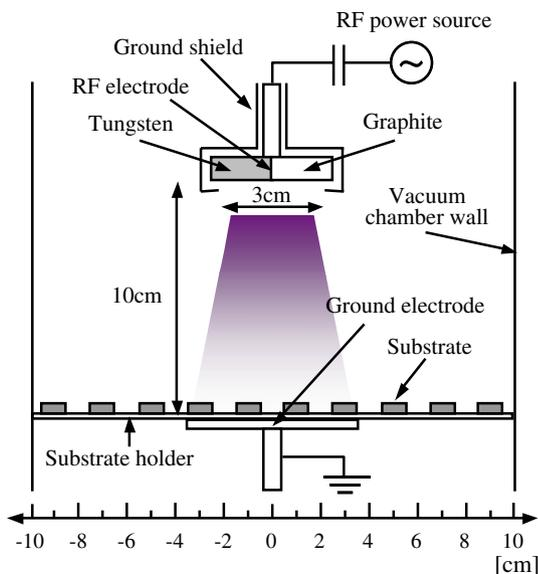
Fig. 1. Installed positions of target and substrates.
