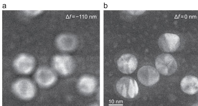
**Fig. 2.** LAADF STEM images of polycrystalline gold nanoparticles on an amorphous carbon film. (a) Images at an underfocus  $\Delta f = -110$  nm showing the presence of halos. (b) In focus images of the same particles ( $\Delta f \approx 0$  nm) show atomic columns and structure due to internal twinning planes is discernible.
