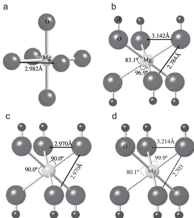
**Fig. 1.** The nearest-neighbor structures around Mg in (a) MgO, (b) Mg(OH)<sub>2</sub>, (c) modified Mg(OH)<sub>2</sub>-I, and (d) Mg(OH)<sub>2</sub>-II. The structure parameters are given in Table 1.
