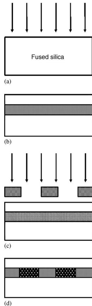
Fig. 1. Manufacturing procedure: (a)  $\text{H}^+$  ion implantation in fused silica, (b) a new waveguide is formed, (c) additional  $\text{He}^+$  implantation with a periodic metal mask covering the surface and (d) grating structures are formed.
