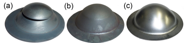
Fig. 4. Hot and cold-stamped cups for s = 40 mm. (a) Hot, v = 26 mm/s, (b) hot, v = 149 mm/s and (c) cold, v = 26 mm/s.
