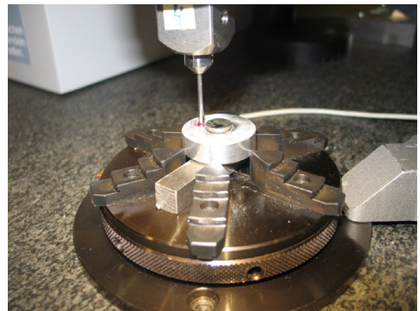
Fig. 2. Specimen on indexing fixture being measured by the 4 mm probe.
