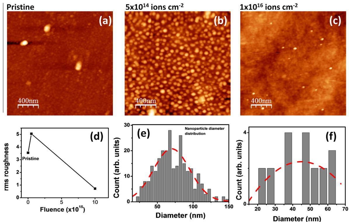
**Fig. 1.** AFM images of the (a) pristine sample and samples irradiated to the fluences of (b)  $5 \times 10^{14}$ , and (c)  $1 \times 10^{16}$  ions  $\text{cm}^{-2}$ , (d) rms roughness of the pristine and irradiated samples, (e) and (f) are diameter distributions of nanodots observed at the fluences of  $5 \times 10^{14}$  and  $1 \times 10^{16}$  ions  $\text{cm}^{-2}$ , respectively. The dashed red lines in (e) and (f) represent the Gaussian fits to the data.
