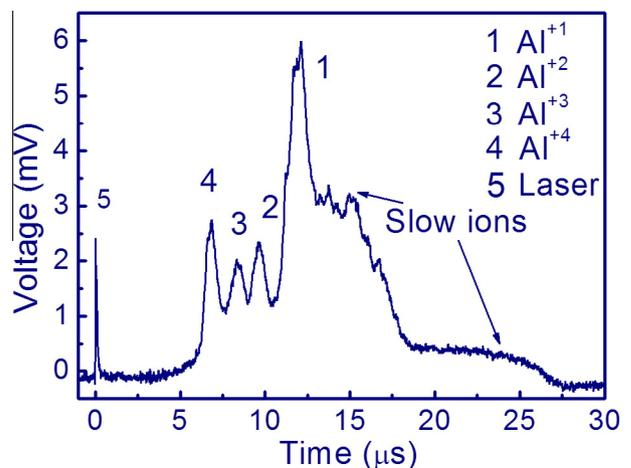
**Fig. 3.** Generation of Al multicharged ions for 5 kV accelerating voltage with a laser pulse energy of 90 mJ shows charge state up to  $\text{Al}^{+4}$ .
