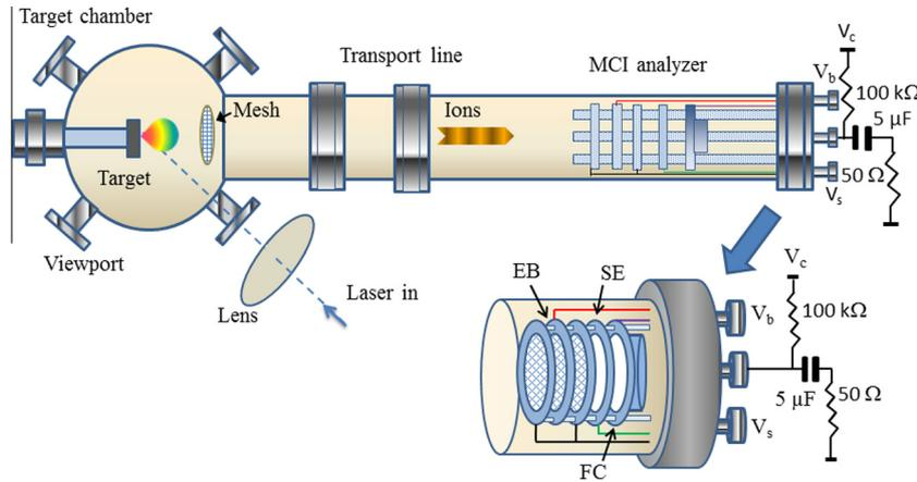
**Fig. 1.** A schematic of the laser multicharged ion source showing the target chamber and the electrostatic time-of-flight energy analyzer, EB: the electrostatic barrier, SE: suppressor electrode, and FC: Faraday cup.
