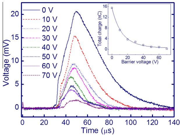
**Fig. 2.** Dependence of the generated multicharged ions on barrier voltage when no accelerating voltage is applied. Inset shows the reduction of total charge with the increase of barrier voltage when no accelerating voltage is applied to the target.
