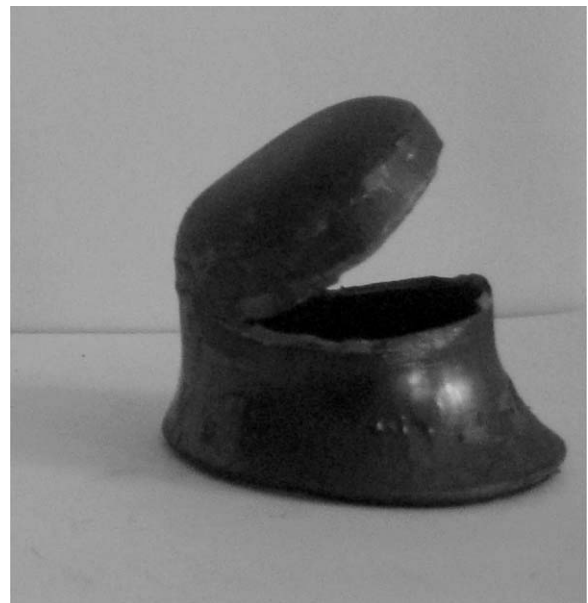
Fig. 3. A typical fracture at 40% reduction.
