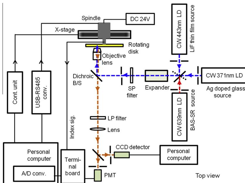
**Fig. 1.** Schematic diagram of a disk-type RPL, PL and PSL readout system (not to scale).
