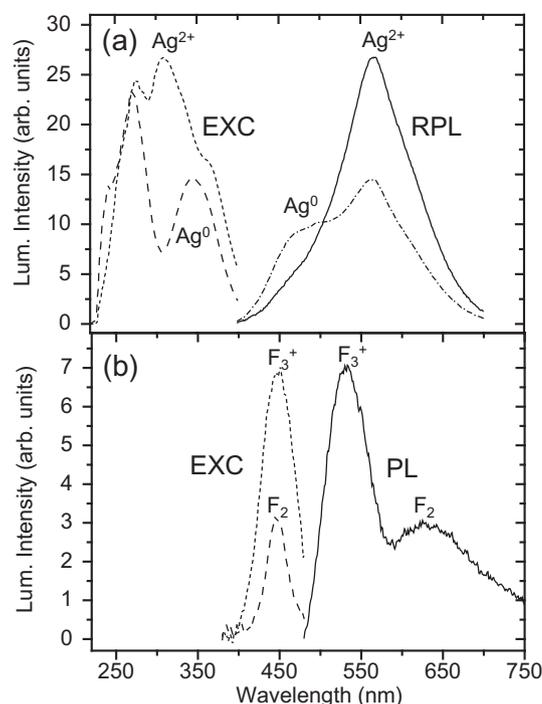
**Fig. 2.** EXC and RPL spectra of Ag-doped glass (a) after X-ray irradiation with an absorbed dose of 1 Gy. EXC and PL spectra of X-ray-irradiated LiF thin films (b) after X-ray irradiation with an absorbed dose of 126 Gy.
