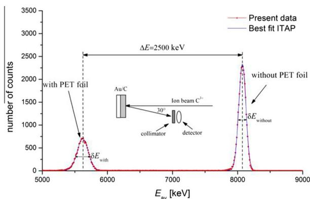
**Fig. 1.** The experimental spectrum of 10.2 MeV C ions backscattered from the Au/C substrate and penetrating the thin PET foil.
