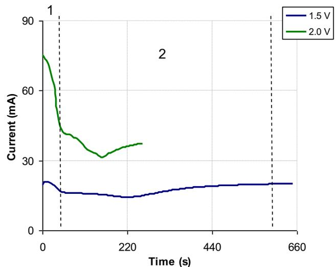
Fig. 1.  $I/t$  curve of Fe/Co nanotube deposition process.
