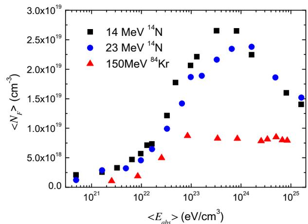
**Fig. 2.** Dependence of the average F-center volume concentration on the average absorbed energy for LiF irradiated with N and Kr ions.
