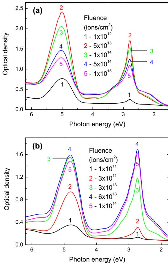
**Fig. 1.** Absorption spectra of LiF crystals irradiated with (a) 14 MeV N ions and (b) 150 MeV Kr ions.
