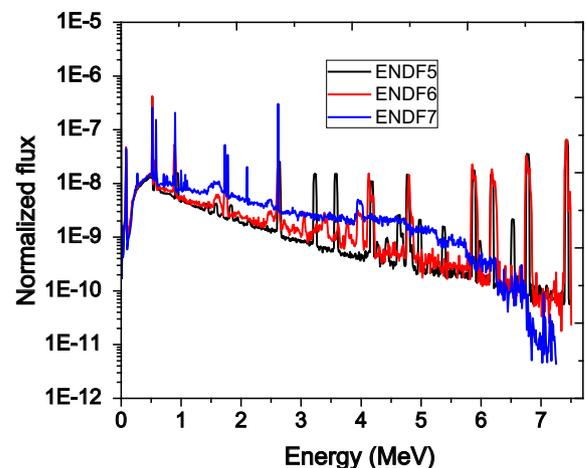
Fig. 3. Gamma ray spectrum in Pb when irradiated with intermediate neutrons.
