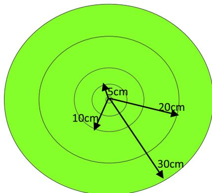
Fig. 1. The spherical model used in MCNP, the tally surface (10 cm radius) can be seen.
