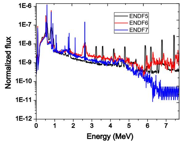
Fig. 2. Gamma ray spectrum in Pb when irradiated with fast neutrons.
