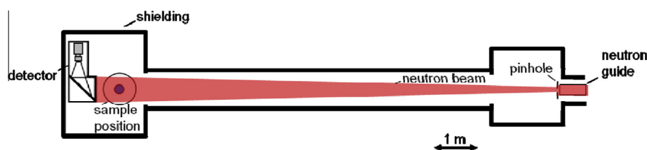
Fig. 2. Layout of the neutron imaging instrument CONRAD-2 (top view). The distance from the aperture to the sample position is 10 m.
