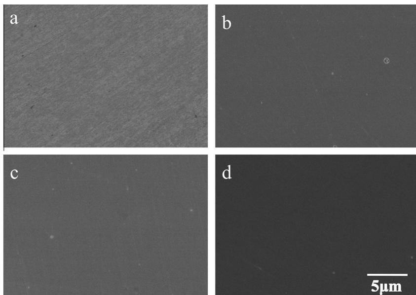
Fig. 1. SEM images of (a) pristine and 500keV  $\text{He}^{2+}$  irradiated  $(\text{Cu}_{47}\text{Zr}_{45}\text{Al}_8)_{98.5}\text{Y}_{1.5}$  with fluences of (b)  $2 \times 10^{17}$  cm<sup>-2</sup>, (c)  $1 \times 10^{18}$  cm<sup>-2</sup> and (d)  $2 \times 10^{18}$  cm<sup>-2</sup>.
