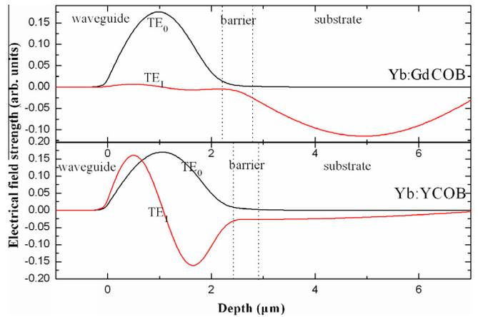
**Fig. 4.** The electrical field intensity distribution of TE modes for Yb: GdCOB and Yb: YCOB waveguides.
