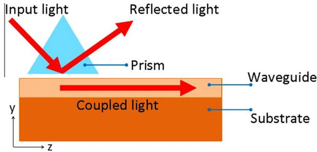
**Fig. 2.** The schematic diagram for prism-coupling experiments.
