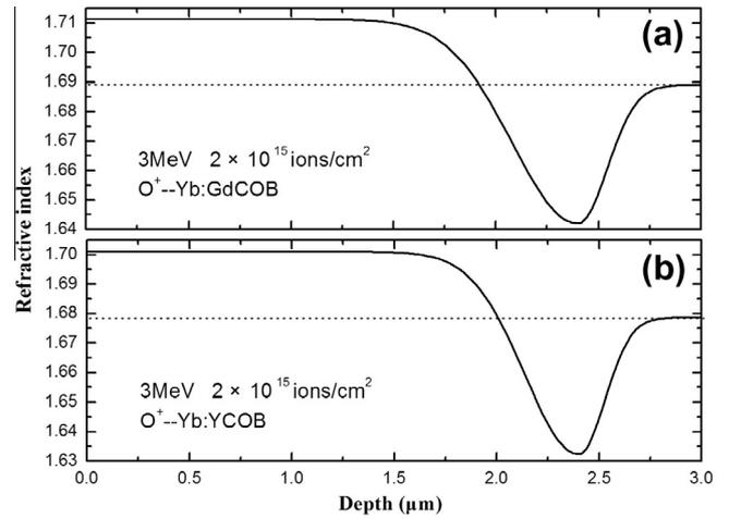
**Fig. 3.** The refractive index ( $n_x$ ) profiles of the (a) Yb:GdCOB and (b) Yb:YCOB waveguides from RCM reconstruction.
