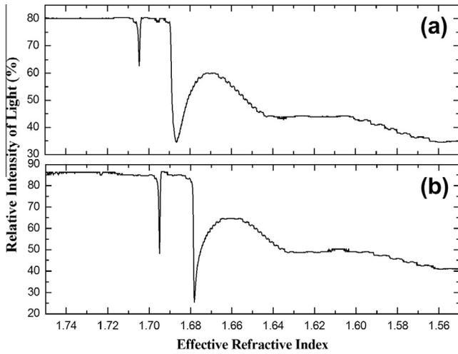
**Fig. 1.** The relative intensity ( $I$ ) of the TE polarized light from the prism vs. the effective refractive index ( $n_{\text{eff}} = n_x$ ) of the incident light for the 3.0 MeV  $2 \times 10^{15}$  ions/cm $^2$   $O^+$  ion-implanted (a) Yb:GdCOB and (b) Yb:YCOB waveguides.
