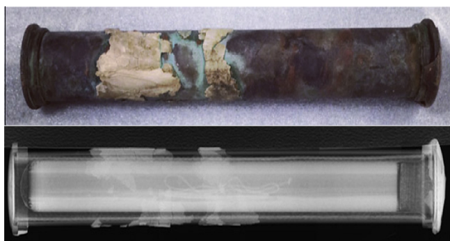
Fig. 2. Time capsule tube (above) and corresponding neutron radiograph image (below).
