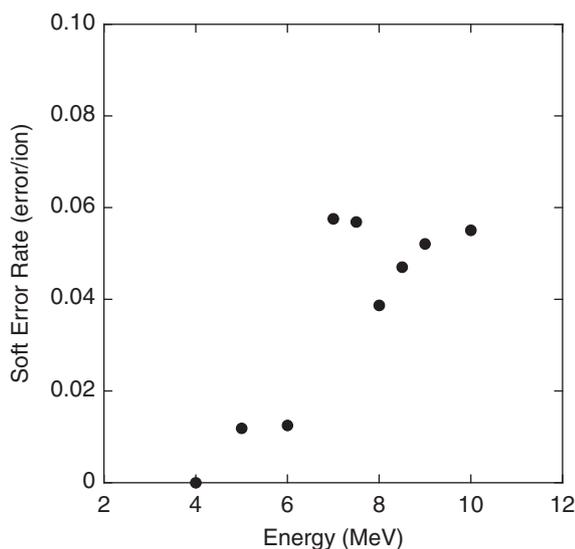
Fig. 1. Soft error rates in the SOI SRAM as a function of beryllium ion energy.
