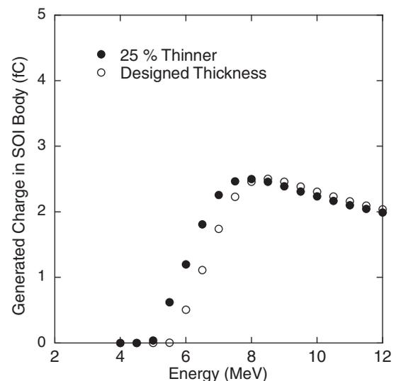
Fig. 2. Generated charges in the SOI body as a function of beryllium ion energy with the designed and 25% thinner over-layer thicknesses.
