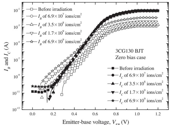
Fig. 3. Variations of collector current ( $I_C$ ) and base current ( $I_B$ ) with emitter-base voltage ( $V_{EB}$ ) for the 3CG130 irradiated by 35 MeV Si ions with different fluences ( $V_{EB} = V_{BC} = 0$  V).
