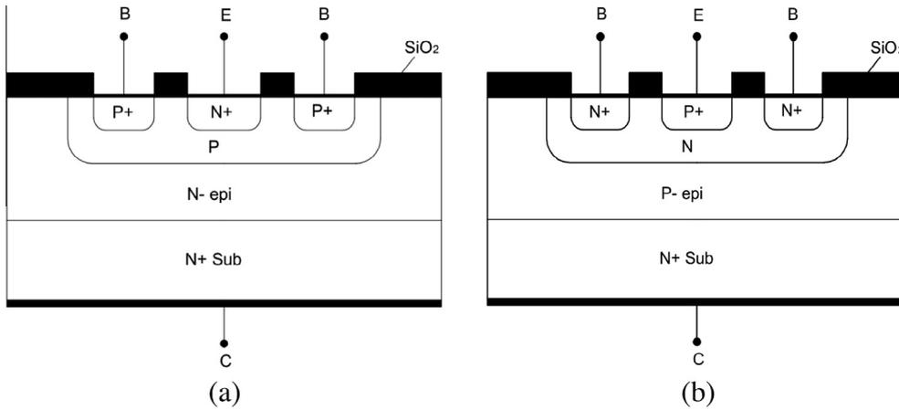
Fig. 1. Cross sections of the bipolar junction transistors: (a) 3DG130 and (b) 3CG130.
