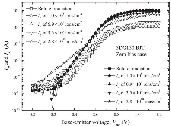
Fig. 2. Variations of collector current ( $I_C$ ) and base current ( $I_B$ ) with base-emitter voltage ( $V_{BE}$ ) for the 3DG130 irradiated by 35 MeV Si ions with different fluences ( $V_{BE} = V_{BC} = 0$  V).
