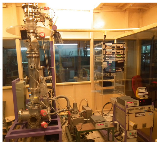
Fig. 1. The completed simple and economic compact ion implanter system at Chiang Mai University. (a) Schematic diagram. (b) Photograph (front view). At the left side is the vertical ion implanter and at the right side is the power supply stack.
