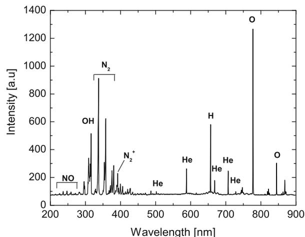
Fig. 4. Emission spectrum of plasma. Plasma power – 34.85 W; He flow rate,  $2.21 \text{ min}^{-1}$ ; axial viewing direction.
