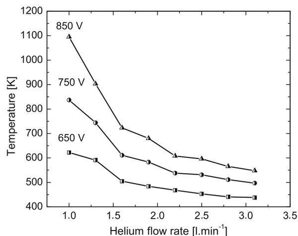
Fig. 3. Dependence of OH rotational temperature on helium flow rate, for different DC supply voltages of the RF generator, in axial viewing direction.
