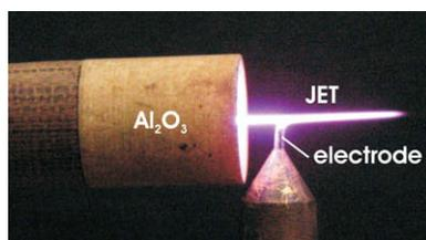
Fig. 2. Photograph of helium plasma jet. Plasma power – 34.85 W; He flow rate –  $2.21 \text{ min}^{-1}$ .
