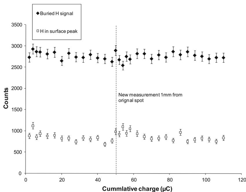
**Fig. 2.** Hydrogen counts in ERDA profile as a function of charge (measurement time). After 50  $\mu$ C of measurement, the analysing beam was moved to a new spot on the sample.
