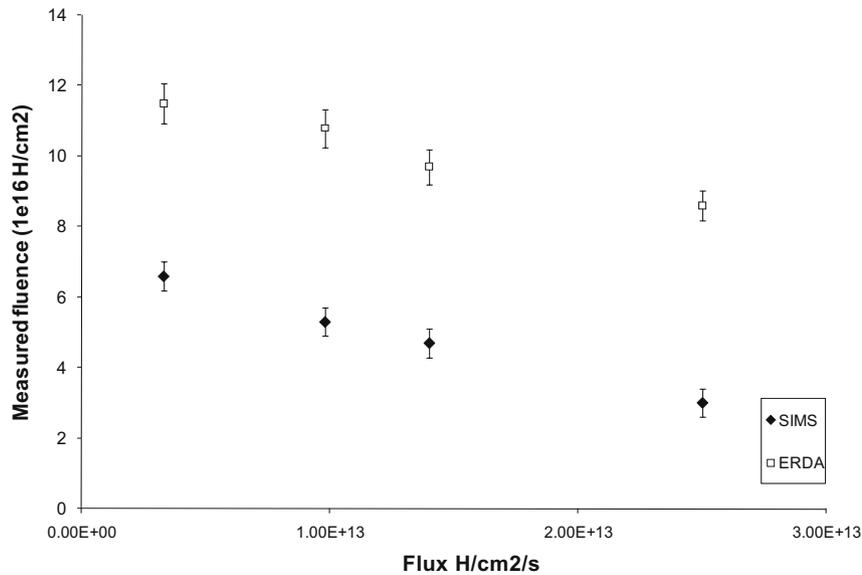
**Fig. 1.** Hydrogen fluence measured by SIMS and ERDA as a function of flux of implanted H, for GaAs wafers implanted  $H_2^+$  with 190 keV at a nominal dose of  $1 \times 10^{17}$  H/cm<sup>2</sup> and at 180 °C.
