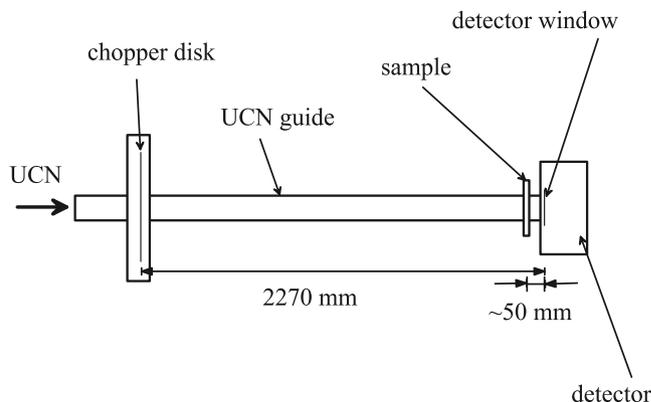
Fig. 1. Sketch of the time-of-flight apparatus.
