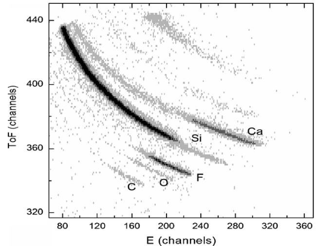
**Fig. 2.** A 2D Time of Flight–Energy mass contour plot showing recoil ions from a  $750 \times 10^{15} \text{ at cm}^{-2}$  (222 nm)  $\text{CaF}_2/\text{Si}$  sample bombarded by 27.5 MeV  $^{84}\text{Kr}$  ions. The contour plot shows O and C impurities present on the sample surface.
