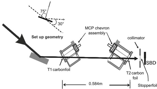
**Fig. 1.** A schematic of the construction of the *ToF-E* spectrometer showing the recoil/scattered ion axis through the carbon-foil based timing detectors T1 and T2 to the stopper foil and the Si SBD. (Not drawn to scale.)
